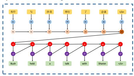
These early models have been greatly improved upon recently through the use of recurrent neural networks organized into an encoder-decoder architecture that allow for variable length input and output sequences. Although effective, the Encoder-Decoder architecture has problems with long sequences of text to be translated. The problem stems from the fixed-length internal representation that must be used to decode each word in the output sequence.
